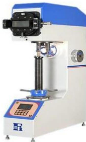
**Figure 4:** The Vickers hardness-testing machine which is used for testing the hardness of the derived samples.
