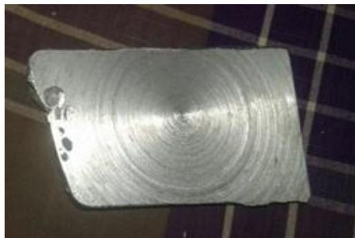
**Figure 3:** The rolled specimen showing the convex shape after rolling.
